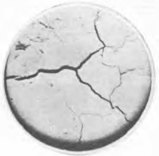
Figure 3. Crack pattern in 'modified oedometer' sample (of black earth) following stress cycle in Figure 10.
