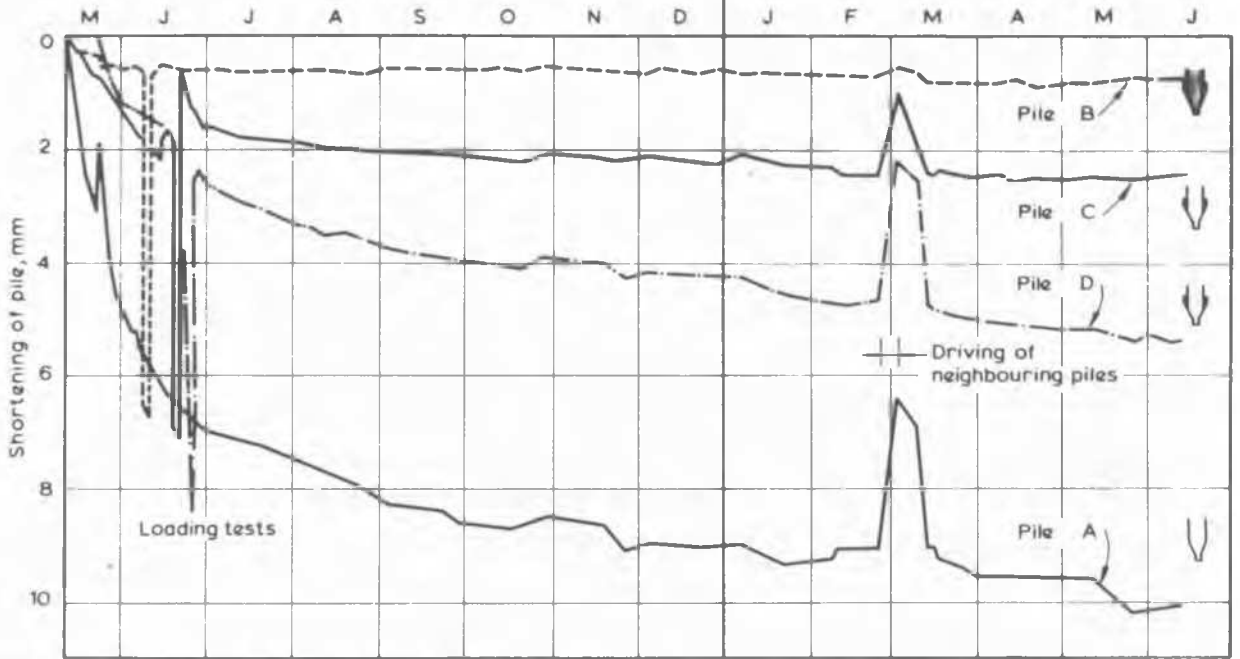
Fig. 4 Total shortening of piles against time.
