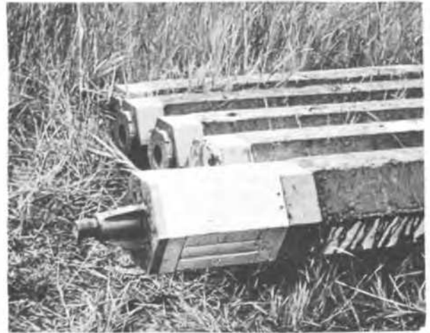
Fig. 2 Photo of pile-force gauge placed at the pile tip. The pile tip is provided with a rock point of hardened steel
