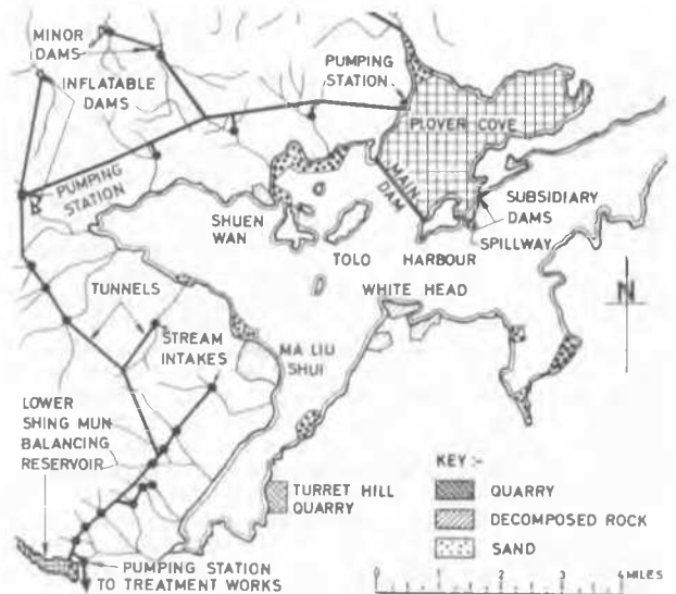
Fig 1 Layout of Plover Cove Water Scheme & Sources of Filling Materials
