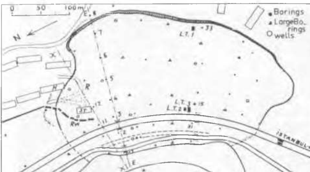
Fig. 3 Plan showing the places of borings and test pits which were converted into observation borings and wells. (L.T.) denotes the locations of the lateral load tests on piles.
