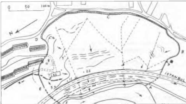
Fig. 2 Plan of the slide area showing the displaced road, septic tank (S.T.), Retaining wall (R.W.), and the tension cracks and wrinkles on the roots and bulged tongues of the slides. Railway track has always been shifted back to its original position following a slide.
