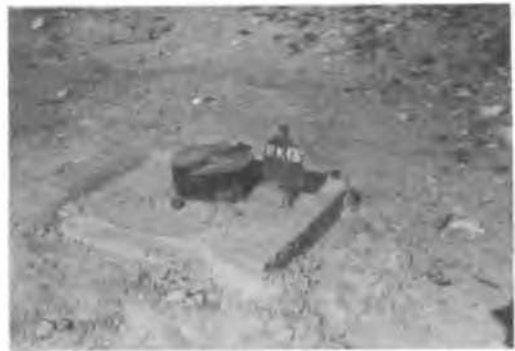
Fig. 4 Head of one of the large diameter observation borings.
