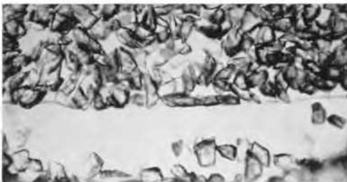
FIG. 2. Microphotograph taken by means of the test set-up shown in Fig. 1. The ice is growing at its upper boundary surface, but the rate of heave of the mineral particles, i.e., the velocity of their upward motion with reference to the ice, is greater than the rate of ice growth, with the result that these particles are accumulated at the ice surface. Magnification about 100 \times .
