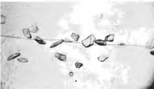
FIG. 4. Microphotograph taken in the same test as that shown in Fig. 3, but about five minutes later. By comparing Figs. 3 and 4, the motions of the mineral particles lying on the ice surface can be observed and measured. The particles which are completely embedded in the ice can be used as fixed reference points. Magnification about 50 \times .
