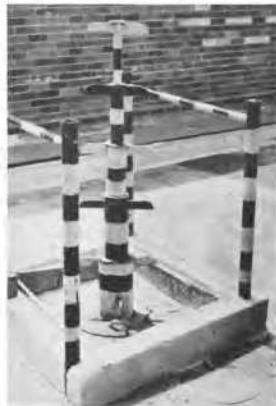
FIG. 7. Surface points in a deep telescopic benchmark.
