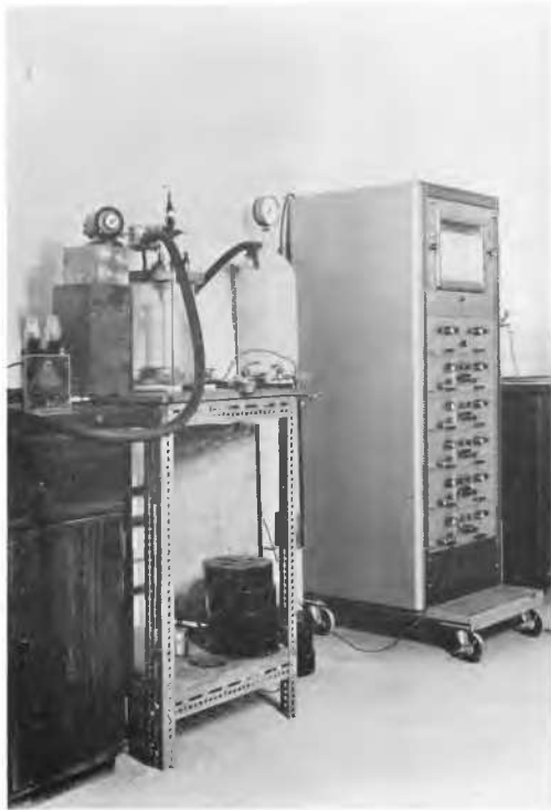
FIG. 3. General view of equipment for deviator stress tests.
