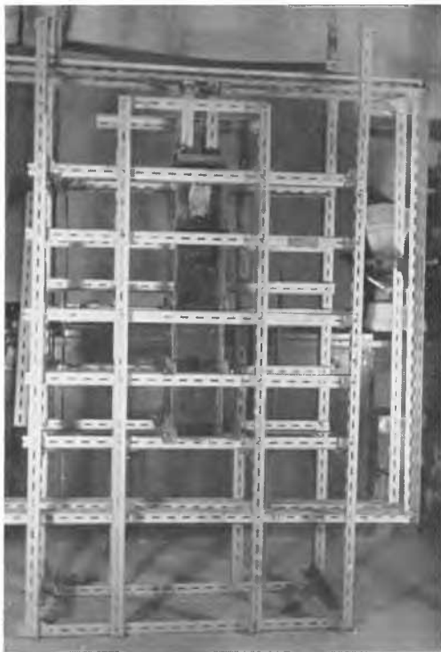
FIG. 1. 1 ft × 6 in. × 3 ft tank used in confined load test.
