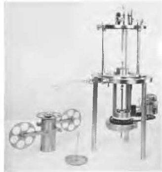
FIG. 1. Photograph of vane-triaxial apparatus and calibration device.
