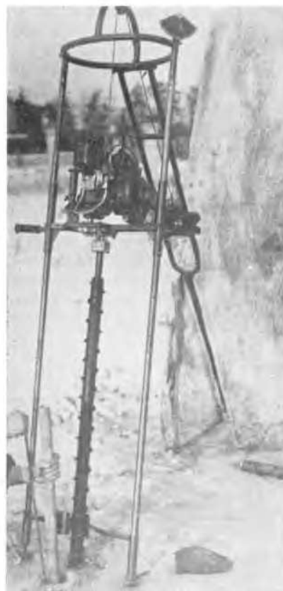
FIG. 4. Extraction of frozen soil core from borehole.
