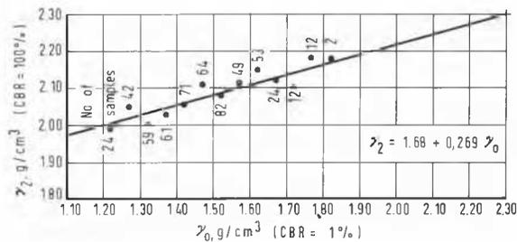
FIG. 3. Correlation between dry densities corresponding to C.B.R. = 1 per cent and C.B.R. = 100 per cent for different soils.
