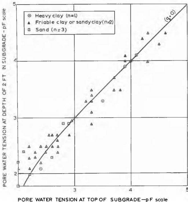
FIG. 1. Comparison of the pore water tension in soil at two different levels under the central part of bituminous-surfaced roads.
