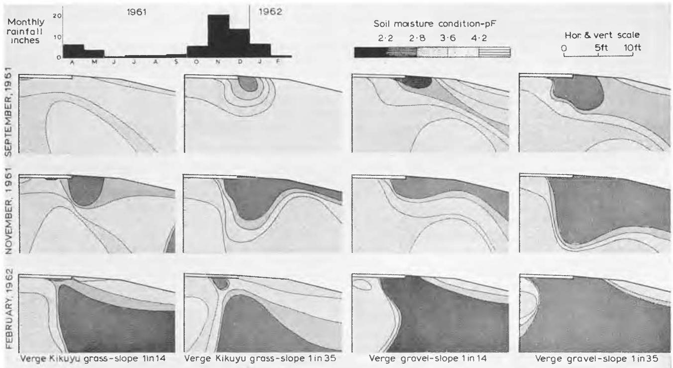
FIG. 2. Effect of verge treatment on moisture conditions at the edge of a road pavement, Muguga, Kenya.
