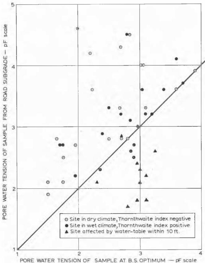
FIG. 4. Comparison of pore water tension in undisturbed samples from road subgrades with that in samples compacted at the optimum moisture content in the British Standard compaction test.
