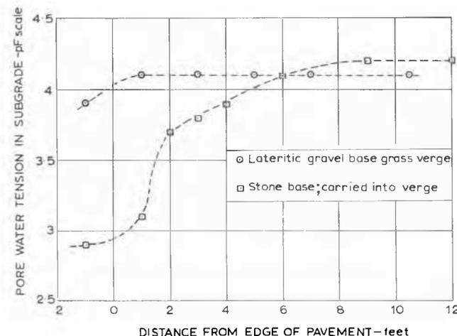
FIG. 3. Effect of base and verge construction on the pore water tension in road subgrades of heavy black clay, Kenya.
