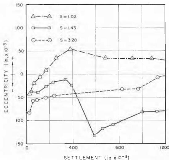
FIG. 9. Experimental variation of eccentricity with settlement.
