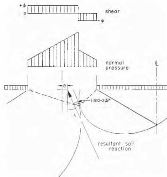
FIG. 2. Method used to calculate forces acting on interfering foundations.
