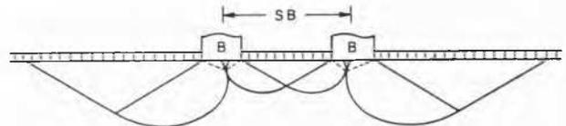
FIG. 1. General interference mechanism for shallow rough based strip foundations.
