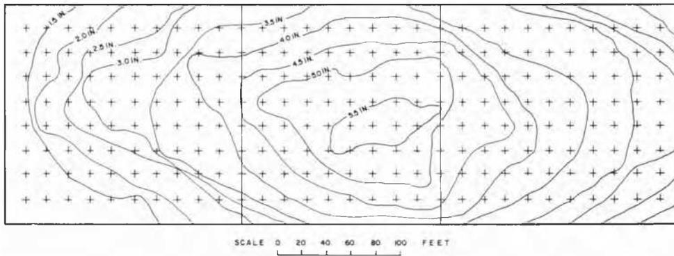
FIG. 1. Contours showing settlement of ground floor.
