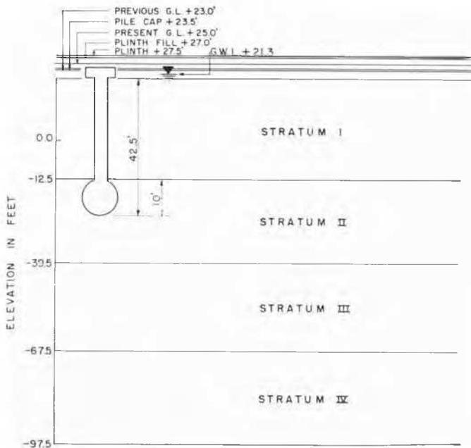
FIG. 2. Cross-section showing various soil strata.
