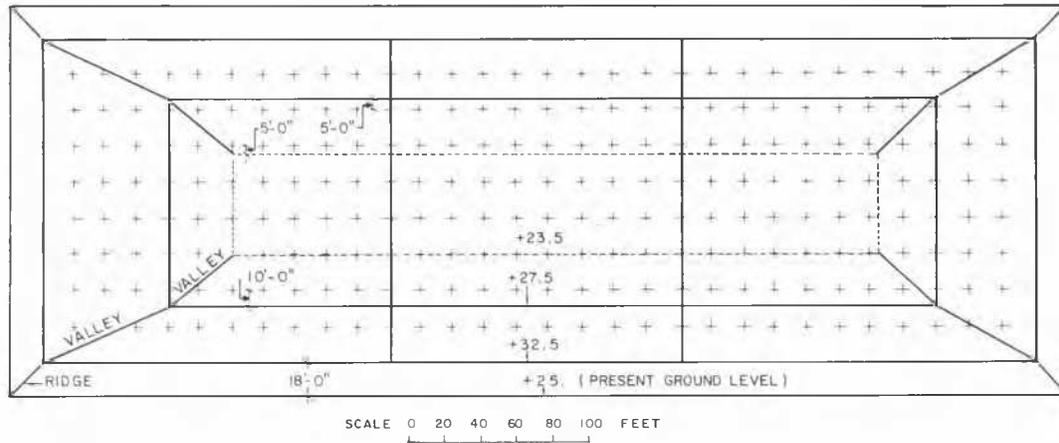
FIG. 4. Filling with soil for reducing differential settlements.
