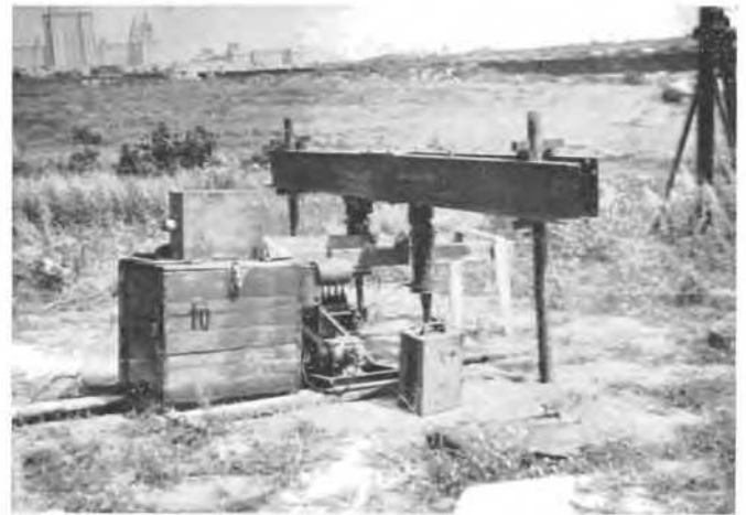
FIG. 2. Testing of probes under static load.
