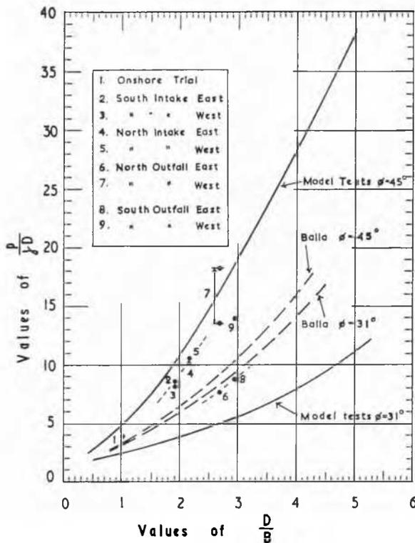
FIG. 3. Comparison of theoretical, model test, and site results.
