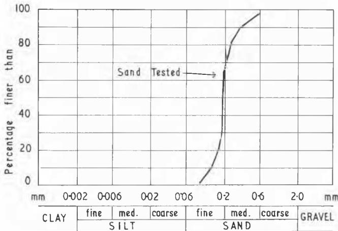
FIG. 1. Particle size distribution of soil tested.
