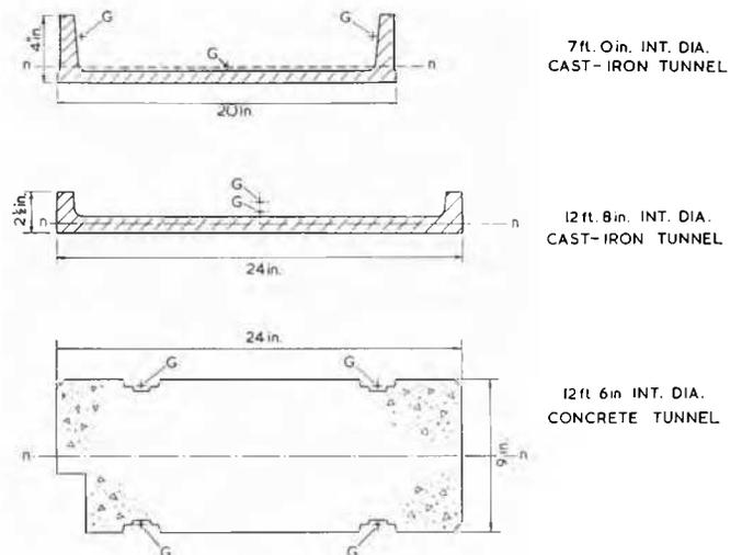
FIG. 1. Radial sections through the lining segments showing positions of gauge wire axes (G) and the neutral surfaces (n n).
