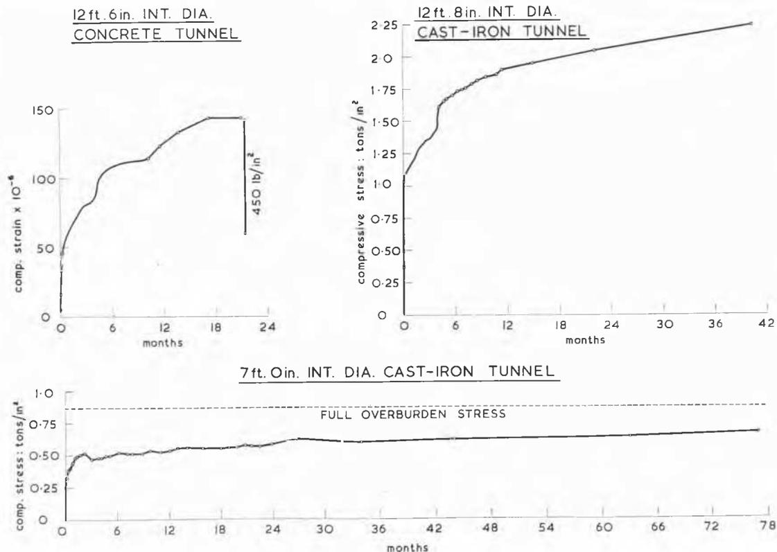
FIG. 3. The development of the average direct stress (or strain) in the three rings with time after construction; the upper two diagrams for Site V and the lower one for Site O.
