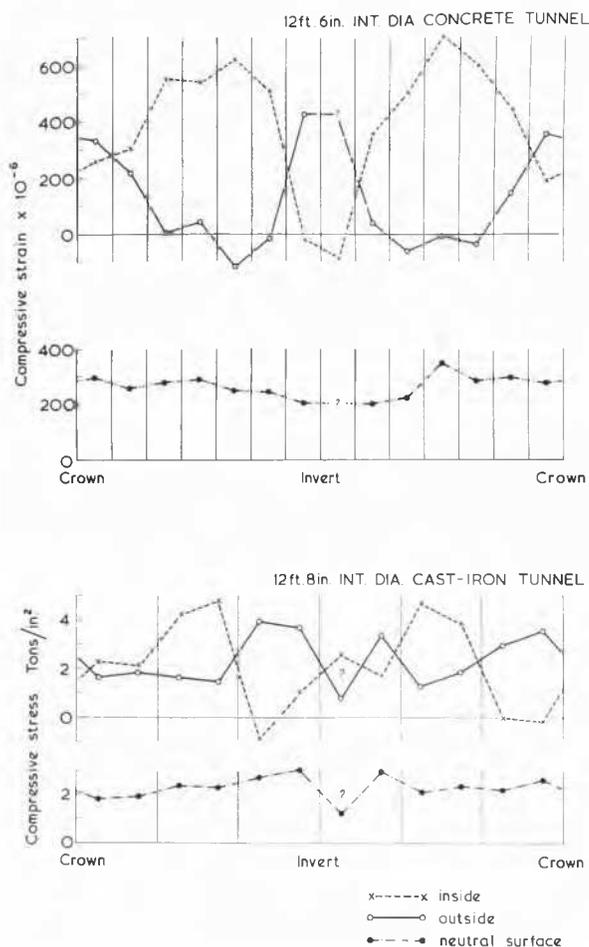
FIG. 4. The distribution of stresses and strains at the inner and outer extremities and at the neutral surface of the segments at Site V.
