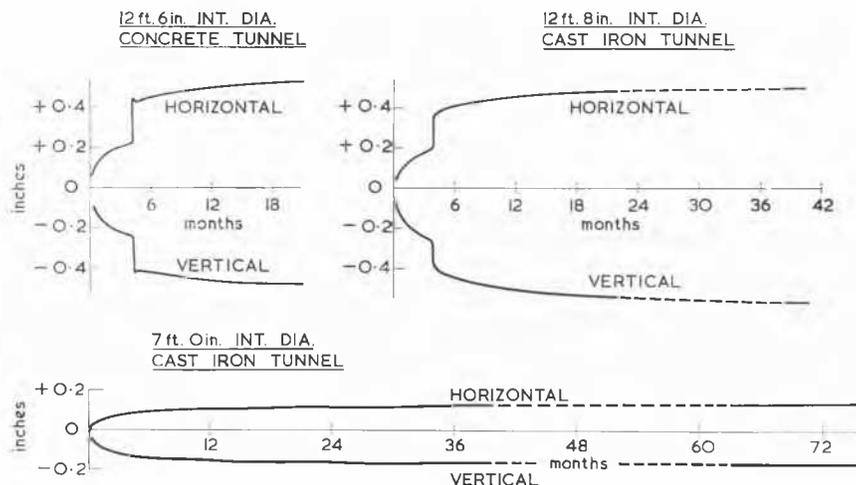
FIG. 2. The changes in horizontal and vertical diameters of the three tunnel linings; the upper two diagrams for Site V and the lower one for Site O.
