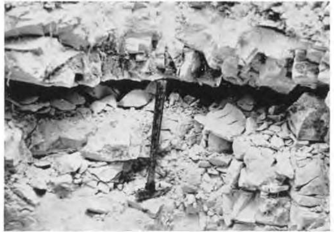
FIG. 4. Wide-open deconsolidation fissure in chalk, 2 m deep in test pit.
