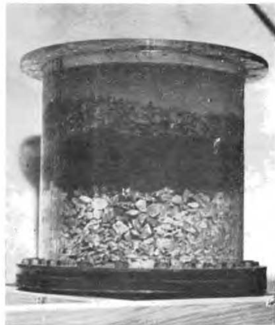
FIG. 2. Photo showing clay, after free swelling, in contact with coarse filter material.
