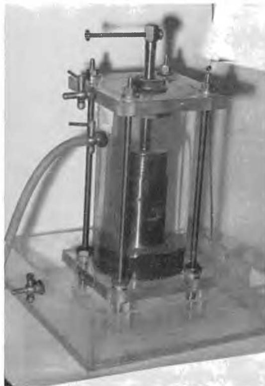
FIG. 4. Photo showing over-all set-up used for model studies of piping in compacted clay.
