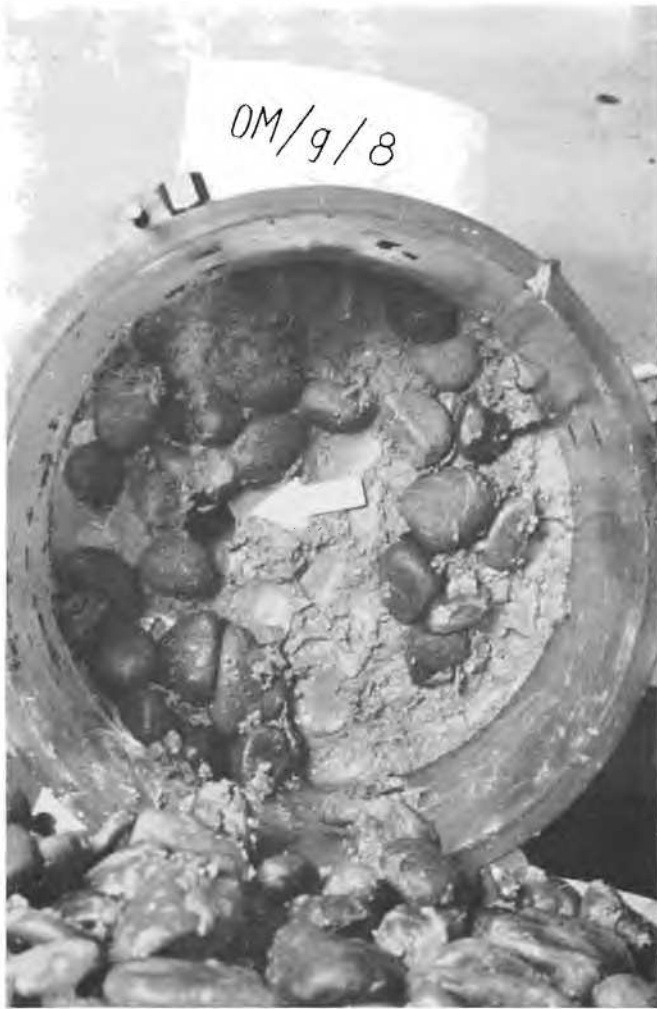
FIG. 4. Contact surface after test, with piping channel.
