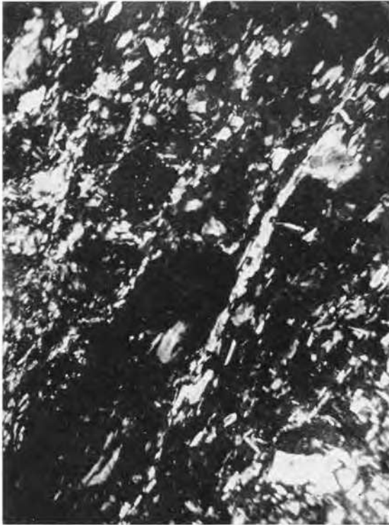
Fig. 2 Microphotograph of a zone of shear in a primary kaolin sample before rupture. A number of orientated clay particles bands is clearly seen. Increase 80 \times .
