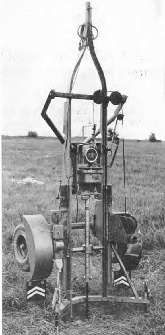
Fig. 1 Asond boring machine during measurement of shear strength. Observe the guiding arrangement with the same pitch as that of the helical point (cf. Fig. 3).
