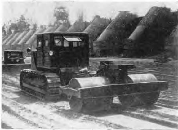
Fig. 4 The vibro-roller PVK-25 (designed by A. A. Smoljar and V. J. Somov).
