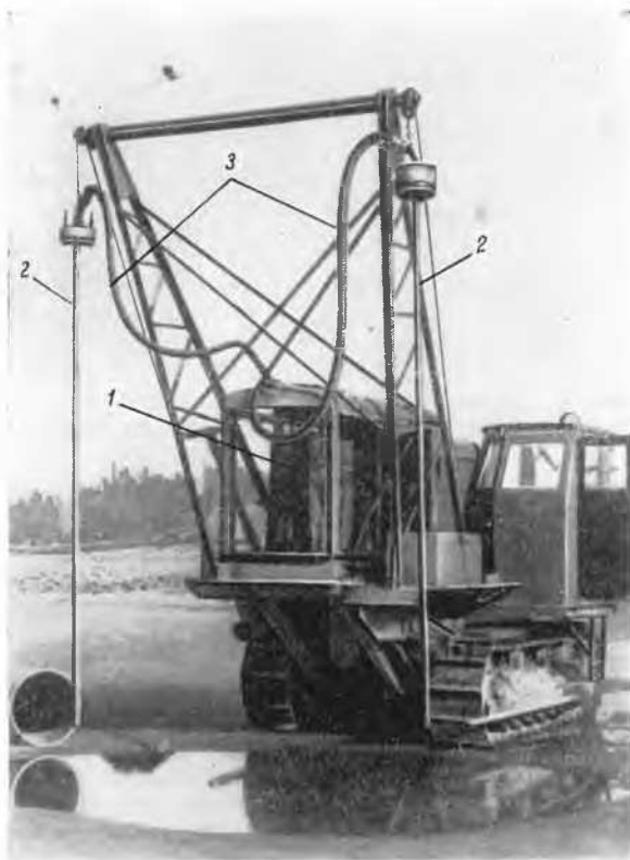
Fig. 5 Compressed air machine for compacting (designed by D. A. Trifonov-Jakovlev).
