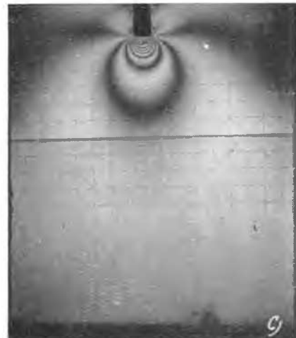
Fig. 5 Isochromatic lines : (a) h = 0 , (b) h = 2b , (c) h = 4b . Les lignes isochromatiques : (a) h = 0 , (b) h = 2b , (c) h = 4b .
