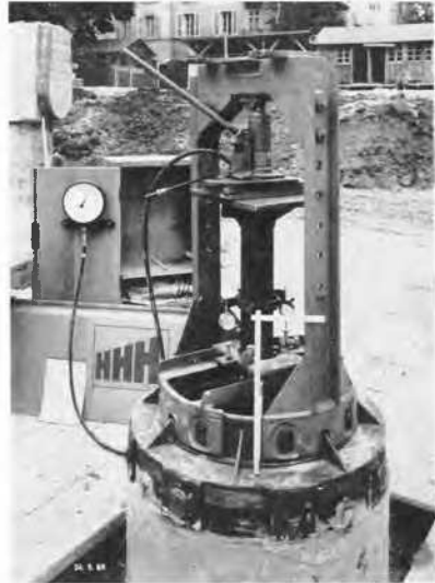
Fig. 6 Testing device of the model pile.
