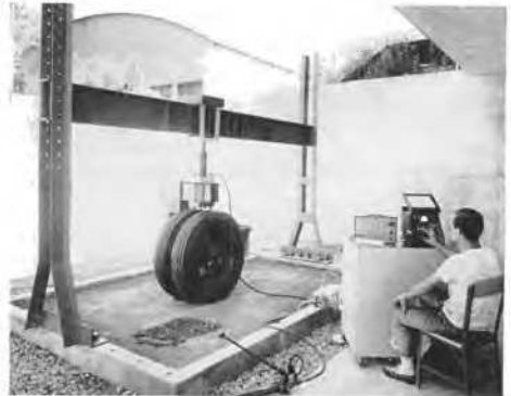
Fig. 3 General view of the model with the loading equipment and strain-measuring apparatus.
