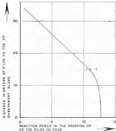
Fig. 8 Horizontal strut reaction related to distance from embankment.
