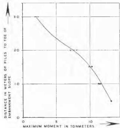
Fig. 7 Bending moments in piles related to distance from embankment.
