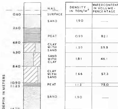
Fig. 1 Boring profile at test site.
