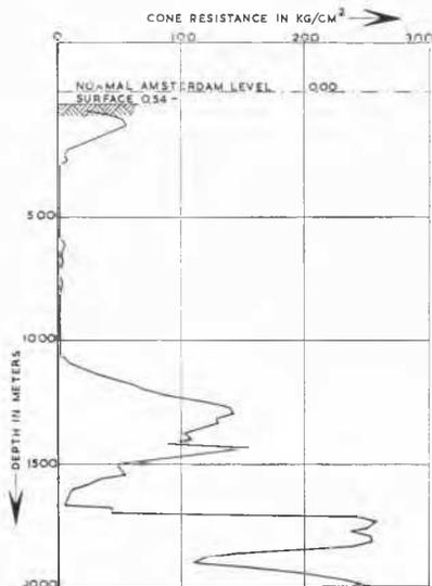
Fig. 2 Cone penetration diagram.
