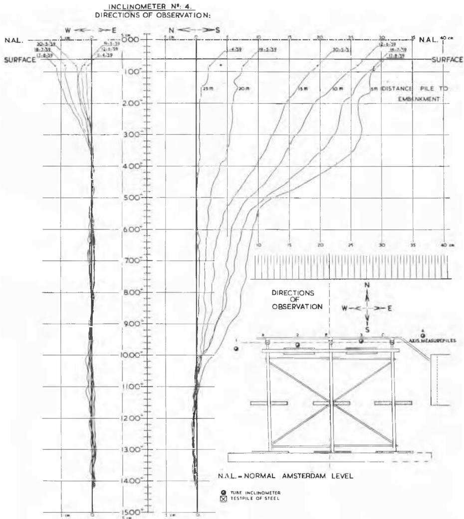
Fig. 9 Horizontal soil displacements measured with inclinometer.
