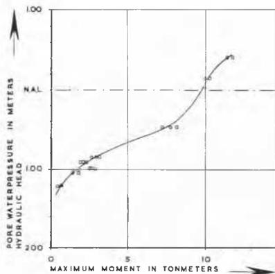
Fig. 10 Maximum bending moment related to pore water pressure in clay layer.
