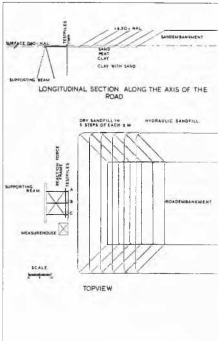
Fig. 5 Schematic plan of tests with steps of embankment extension.
