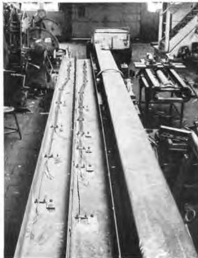
Fig. 3 Test pile with strain gauges during fabrication.
