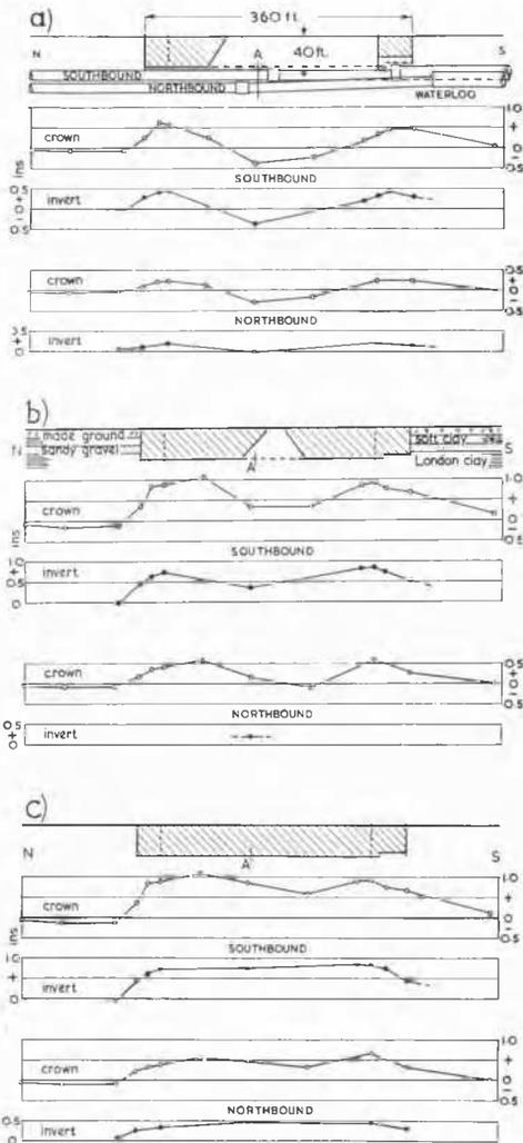
Fig. 2 Sections across the site along the line of the tunnels, showing the state of excavation and the vertical displacements of the crown and invert of both tunnels at three stages a), b) and c).
