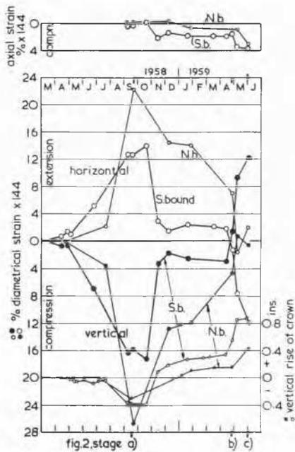
Fig. 3 Movement at the vertical section A in Fig. 2. *Upper diagram.* The variation of axial strain in the north and southbound tunnels as excavation proceeded. *Lower diagram.* The variations of horizontal and vertical diametrical strains and of vertical displacements of the crown of the north and southbound tunnels as excavations proceeded.
