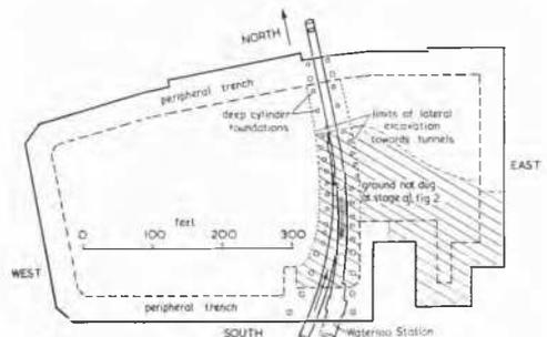
Fig. 1 Plan of site; the whole area was excavated to a depth of about 40 feet.
