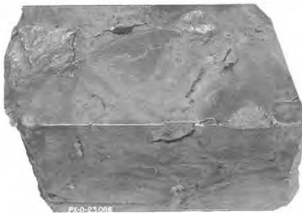
Fig. 16 Oblique view of the undisturbed sample showing the cylindrical failure surface formed by the vane shear test.
