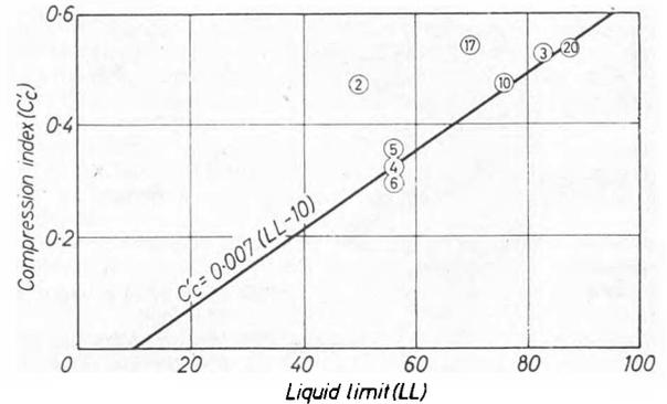
Fig. 5 Compression index versus liquid limit
