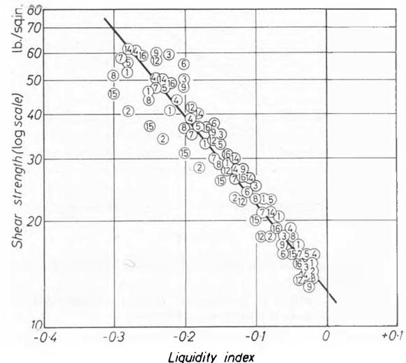
Fig. 3 Shear strength versus liquidity index
