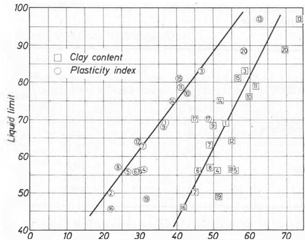
Fig. 2 Liquid limit versus clay content and plasticity index
