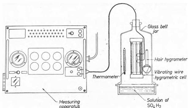
Fig. 5 Schematic drawing of the arrangement used in the calibration of the vibrating wire hygrometric cell
