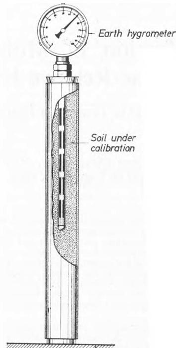
Fig. 3 Arrangement for direct measurement of relative humidity of a soil by an earth hygrometer
