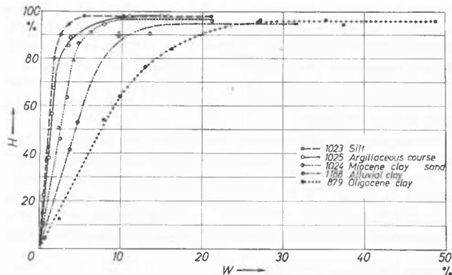
Fig. 2 Relation between the relative humidity ( $H\%$ ) determined with an earth-hygrometer and the moisture content ( $W\%$ ) of 5 Lisbon soils
