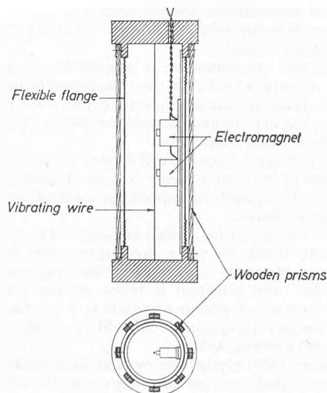
Fig. 4 Schematic drawing of the vibration wire hygrometric cell (in study)
