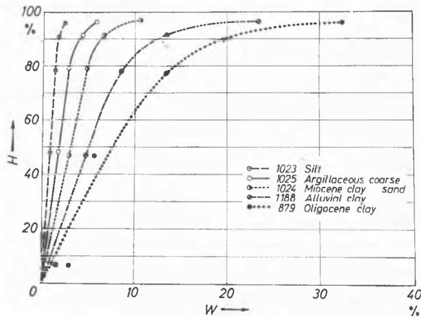
Fig. 1 Vapour pressure curves of 5 Lisbon soils
