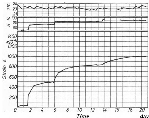
Fig. 6 Results of the calibration test. Strain ( $\epsilon$ ), relative humidity ( $H\%$ ) and temperature ( $t^\circ\text{C}$ ) as a function of time (days)
