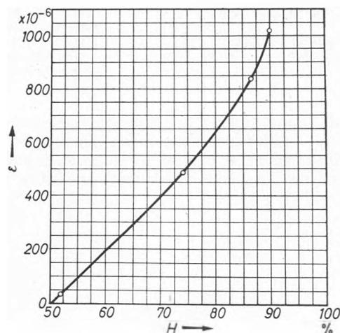
Fig. 7 Calibration curve of the vibrating wire hygrometric cell (relative humidity ( $H\%$ )—strain ( $\epsilon$ ))
