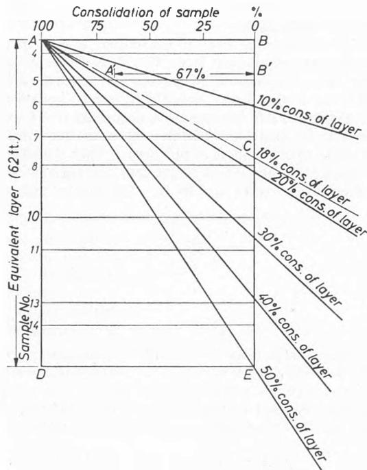
Fig. 3 Approximate method for computing  $U_v$  of individual samples corresponding to given  $U_v$  values of entire layer
