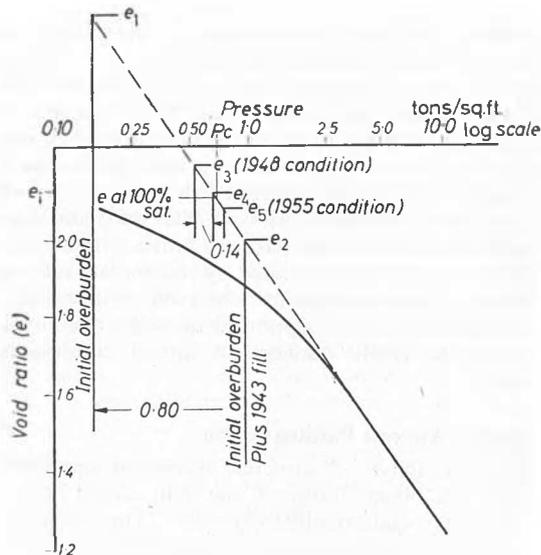
Fig. 2 Typical consolidation test curve
