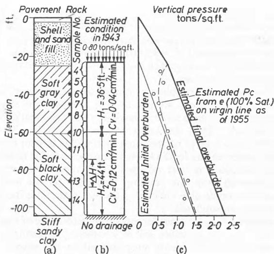
Fig. 1 Typical boring log and pressure diagram
