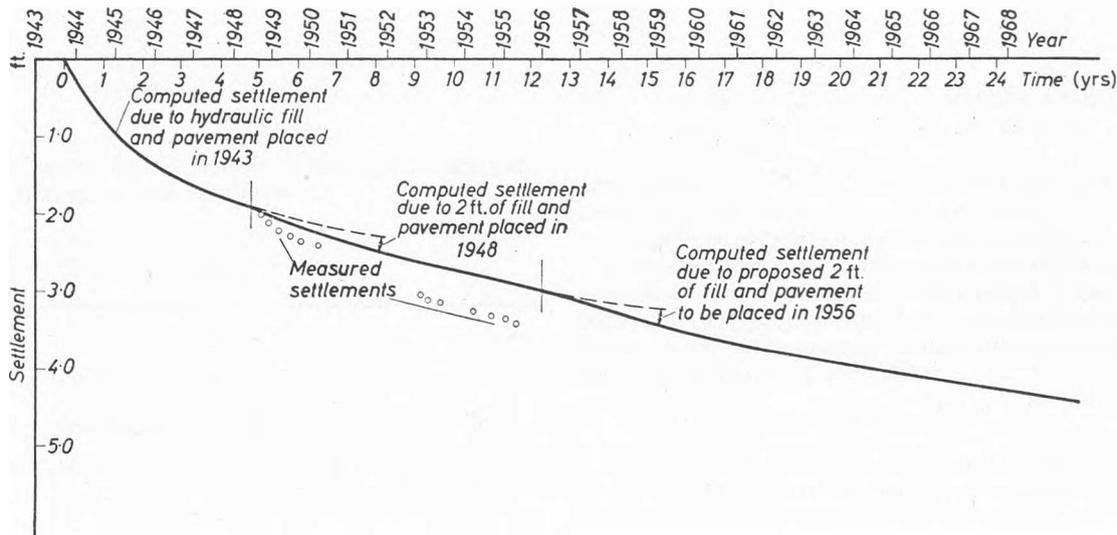
Fig. 4 Composite time-settlement curve
