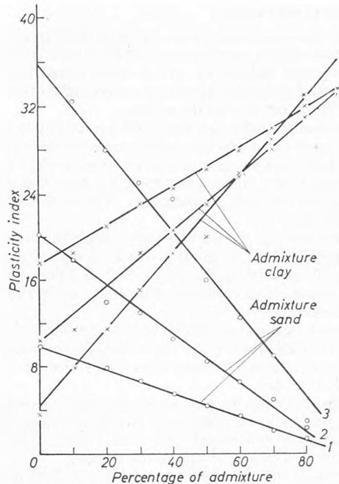
Fig. 2 Relation between plasticity index and percentage of admixture in six typical cases
