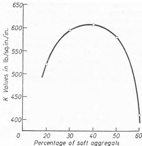
Fig. 1 Relation between percentage of soft aggregate in the upper course of a stabilized soil road crust and the K value in a plate bearing test
