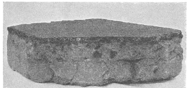
Fig. 3 A section cut from the treated surface after 11 years of service
