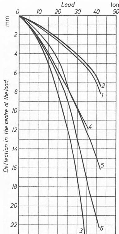
Fig. 5 Loading tests on the runway constructions
