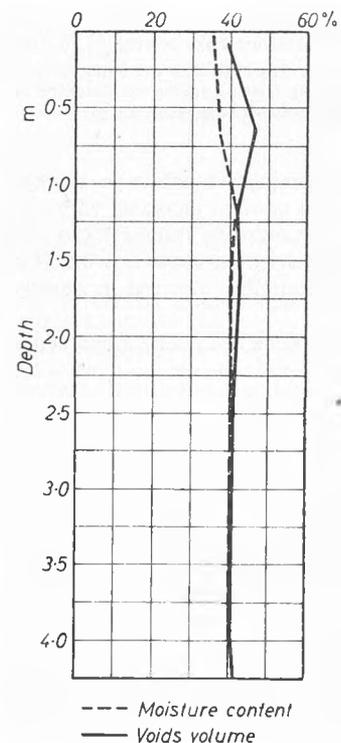
Fig. 2 Measured voids volume and water contents
