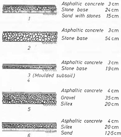
Fig. 4 Types of construction tested
