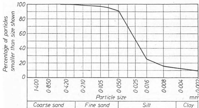
Fig. 1 Grain size distribution curve of the Beek loess
