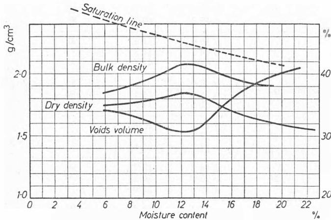
Fig. 3 The result of a compaction test
