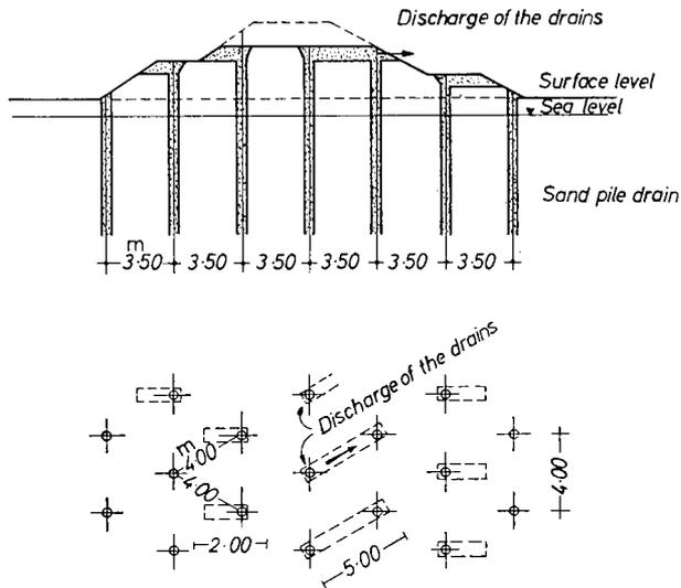
Fig. 7 Arrangement for the discharge of water when the drains have been built in partially constructed levee
