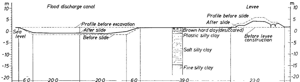
Fig. 2 Cross-section of the first slide and summary of soil profile
