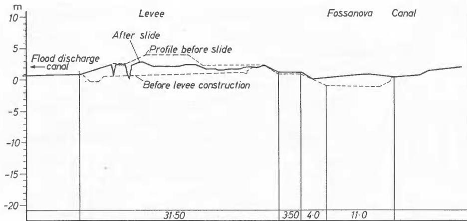
Fig. 3 Cross-section of the second slide
