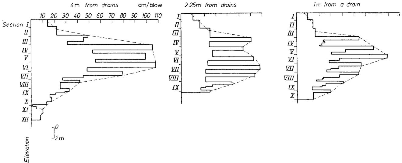
Fig. 6 Penetrometer diagrams after 45 days of drainage at various distances from the drains
