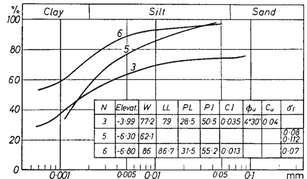
Fig. 1 Grain size curves of some samples and their index properties
