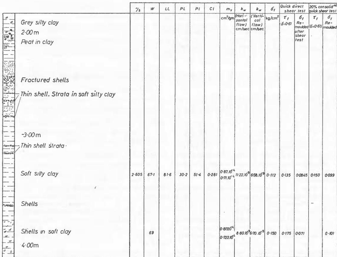
Fig. 4 Cross-section showing the position of shell lenses in the soft silty clay and the laboratory tests carried out on the most important samples
