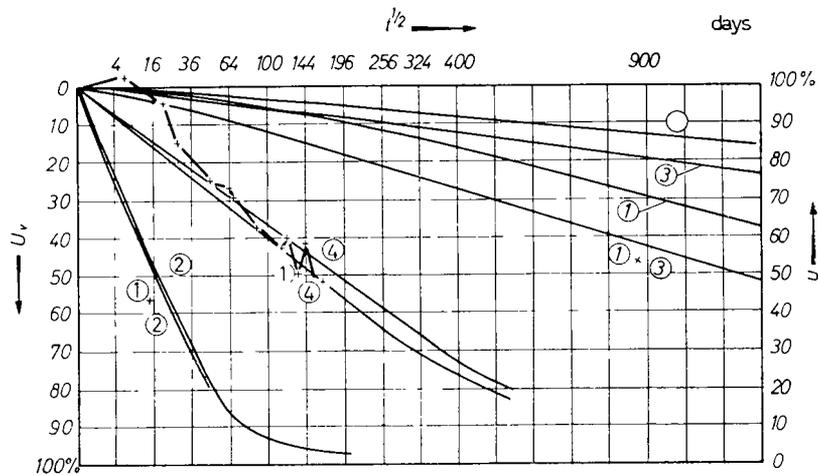
Fig. 5 Relation between per cent consolidation and  $t^{1/2}$  with various thicknesses of impervious soil and comparison with actual consolidation
