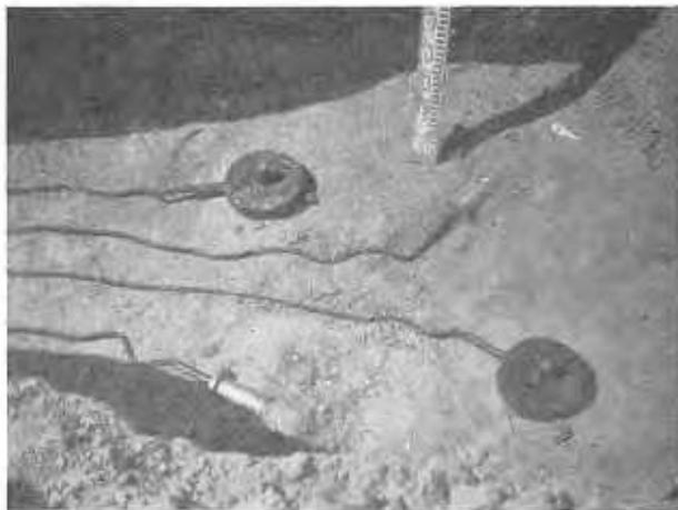
Fig. 5 Details of piezometer and earth pressure cells in the core
