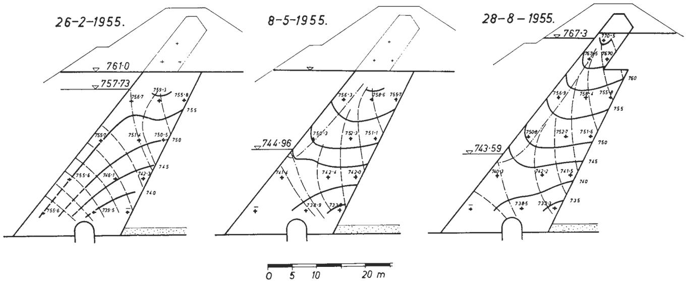
Fig. 6 Measured flow nets—Lokvarka dam
