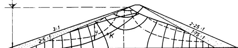
Fig. 9 Theoretical flow nets—dam with wide core
