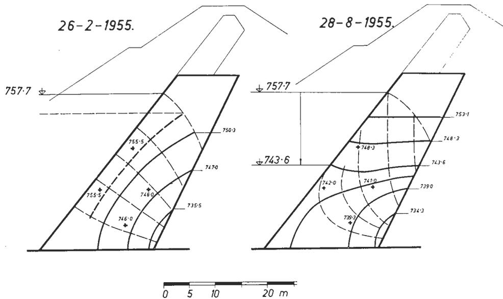
Fig. 7 Theoretical flow nets—Lokvarka dam
