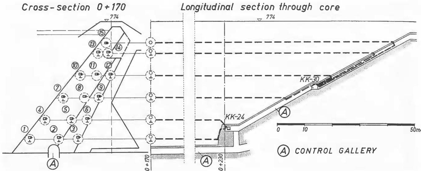
Fig. 4 Locations of piezometers in the core
