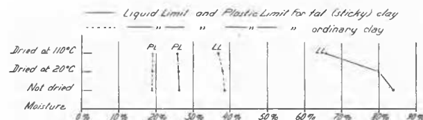
Fig. 2 Average Results on Plastic Limit and Liquid Limit of Sticky and Usual Norwegian Clays in Relation to the Degree of drying out to which the Clays have been Subject before Testing
