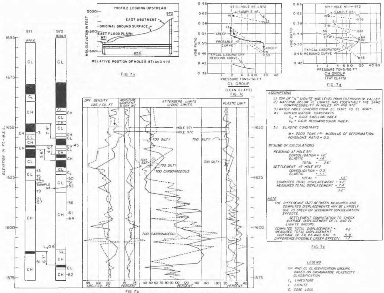
Fig. 7 Studies of the Effect of Unloading in the East Abutment
