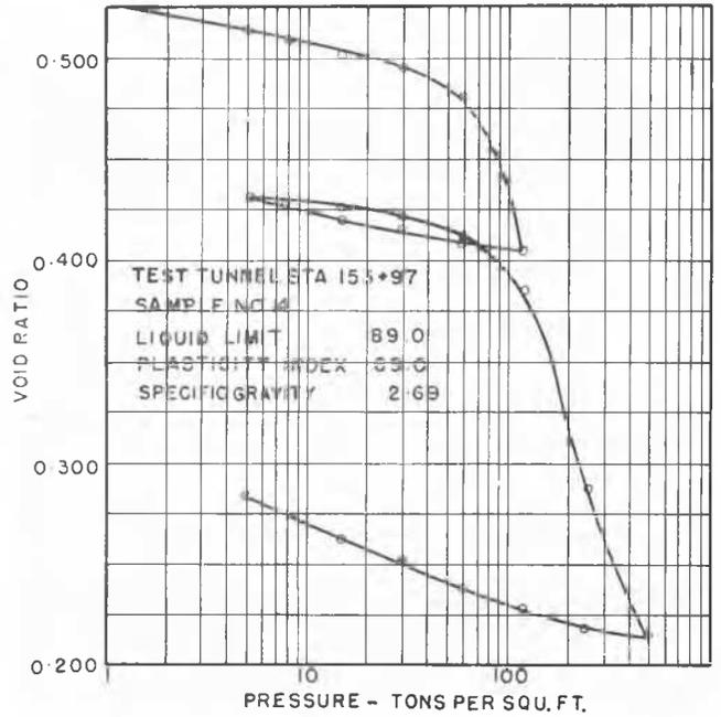
Fig. 5 Typical Result of a Loading Test
