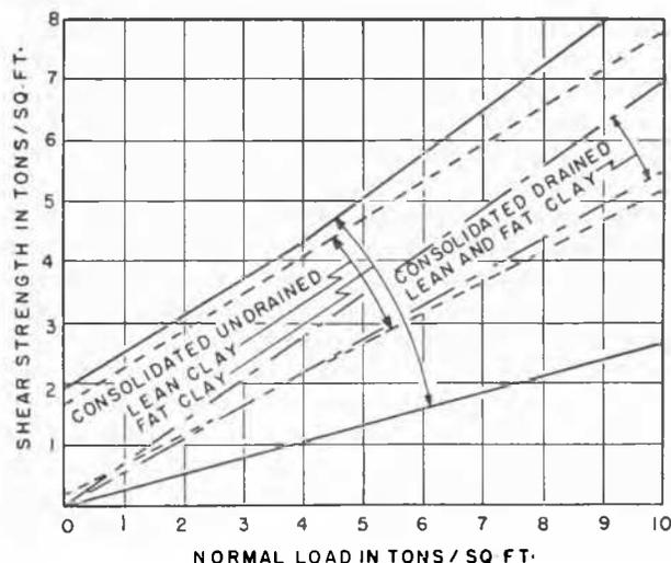
Fig. 3 Results of Direct Shear Tests
