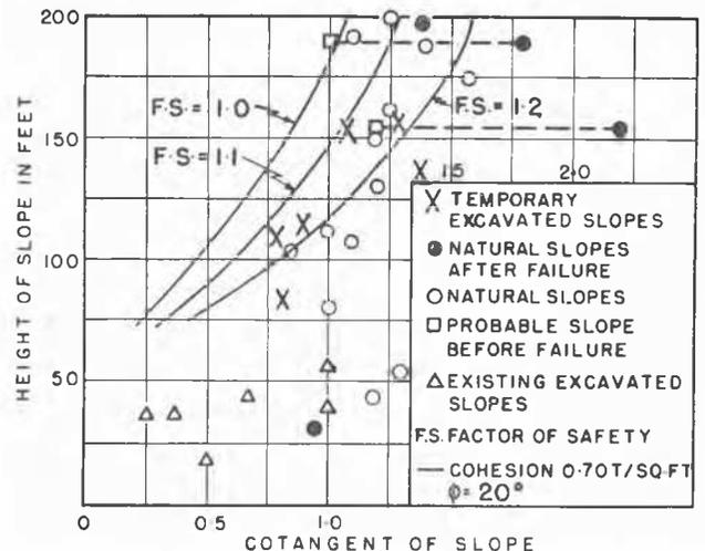
Fig. 6 Field Slope Chart
