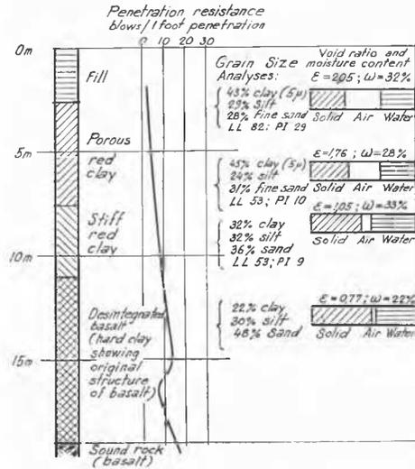
Fig. 2 Soil Profiles in Desintegrated Basalt
