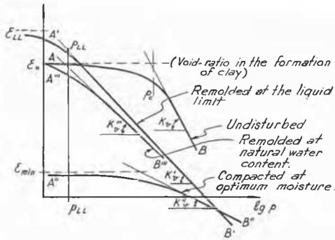
Fig. 7 Consolidation Curves for Residual Clays
