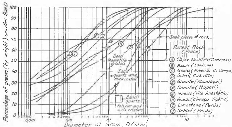
Fig. 3 Grain Size Distribution of Residual Clays
