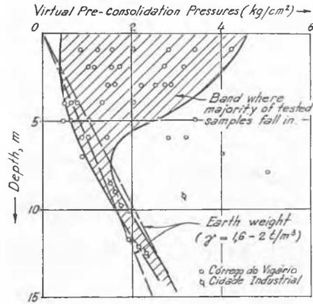
Fig. 8 Virtual Pre-Consolidation Pressures Against Depth of Samples
