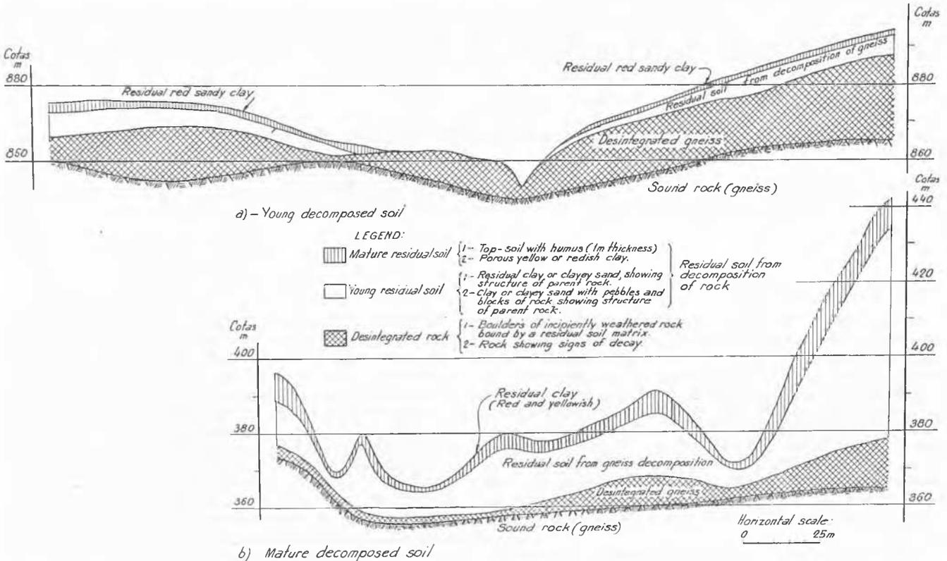
Fig. 1 Cross-Sections through Decomposed Gneiss
