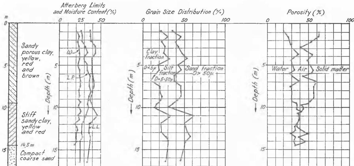
Fig. 5 Porous Residual Clay (Campinas) from Decomposition of a Clayey Sandstone. Variation of Consistence, Grain-Size Distribution and Porosity with Depth
