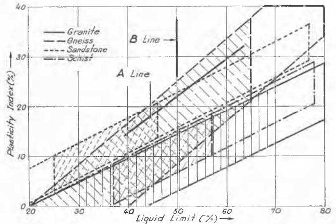
Fig. 4 Residual Porous Clays—Plasticity Chart
