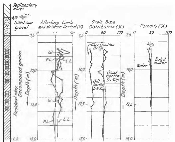
Fig. 6 Residual Clay (Belo Horizonte) from Decomposition of Gneiss. Variation of Consistence, Grain-Size Distribution and Porosity with Depth
