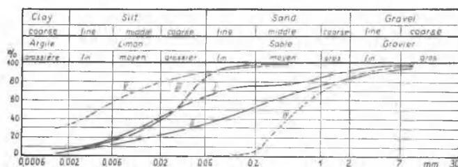
Fig. 1 Grain Size Distribution Curves on Various Kinds of Soil Treated by the New Process and of the Ground Clay Used for the Purpose:
