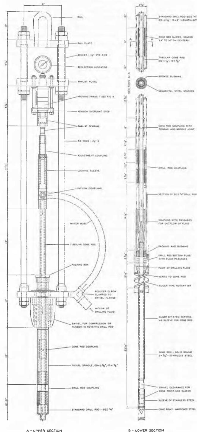
Fig. 2 General Assembly of Penetrometer
