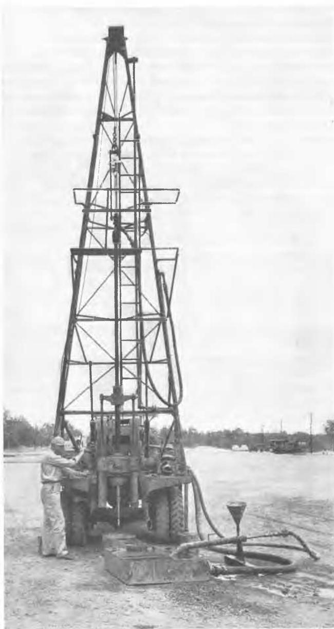
Fig. 1 Rotary Drilling Rig with Penetrometer
