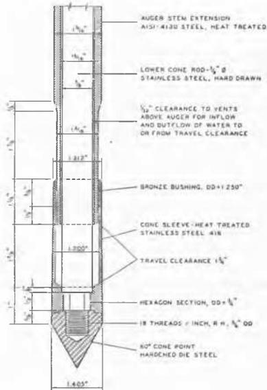
Fig. 3 Details of Conical Point
