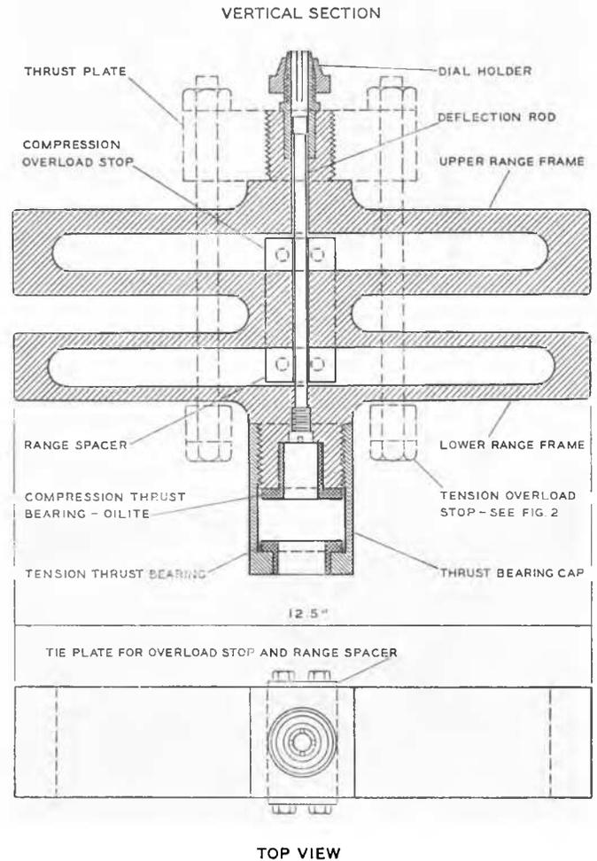
Fig. 4 Double Range Proving Frame
