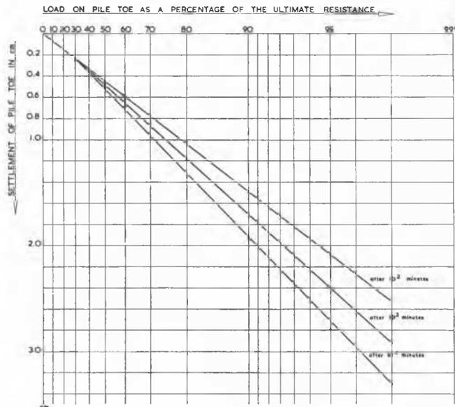
Fig. 8 Load-Settlement Curve of Concrete Pile No. 2, Slotermeer, at Different Time Intervals, Plotted on a Semi-Logarithmic Scale
