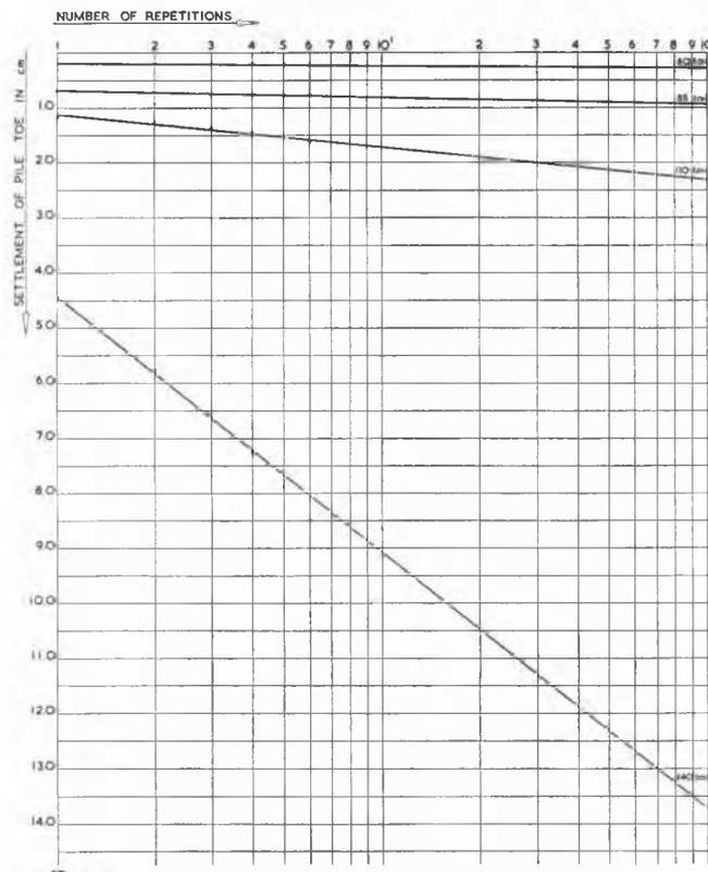
Fig. 9 Semi-Logarithmic Representation of the Influence of Repeated Loading and Unloading of Concrete Pile No. 2, Slotermeer
