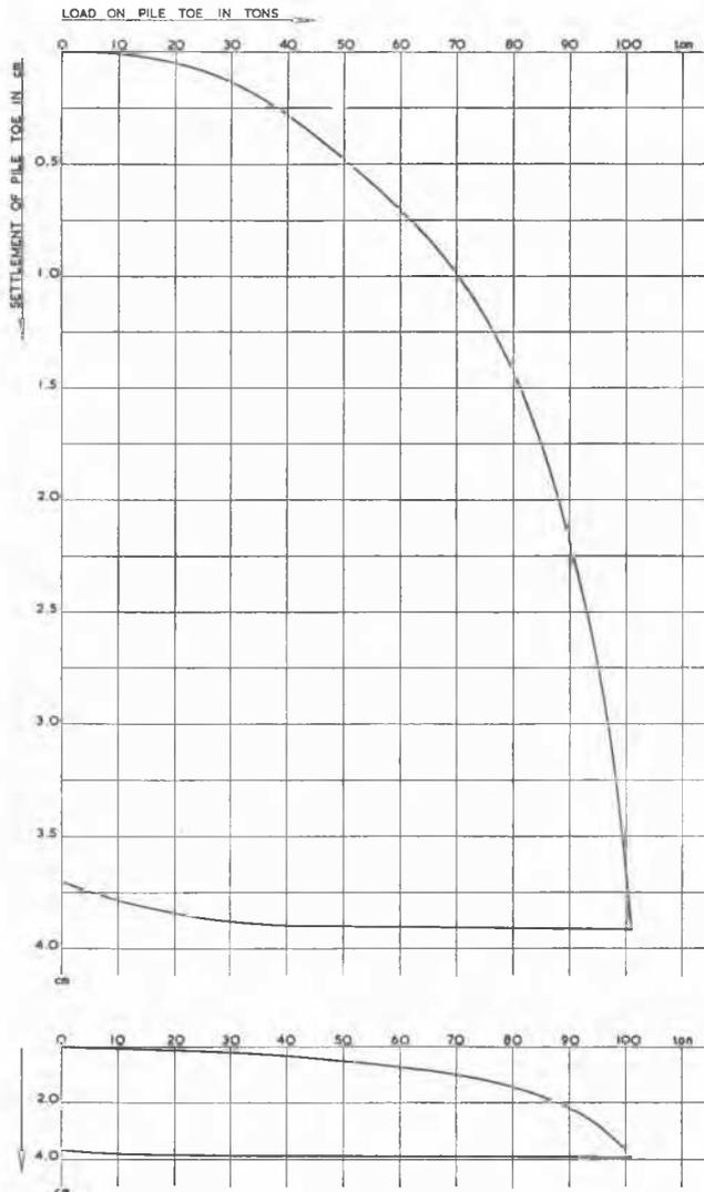
Fig. 1 Load-Settlement Curve of a Concrete Pile in the Harbour Area of Amsterdam
