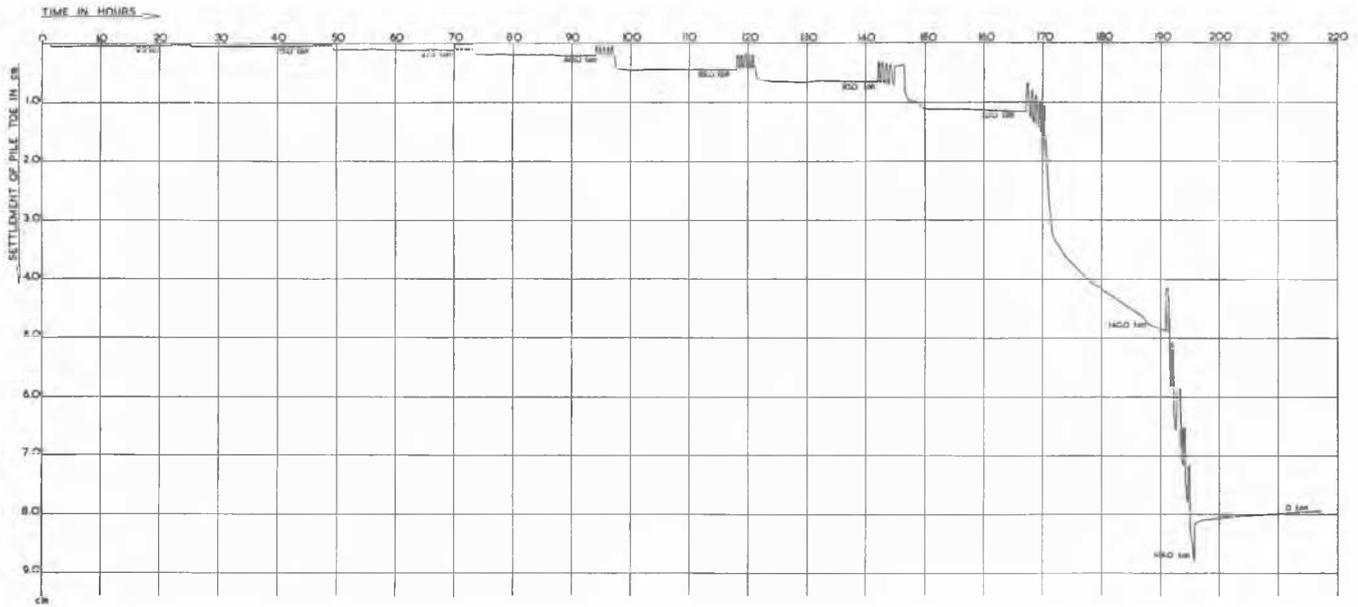
Fig. 5 Time-Settlement Curve of Concrete Pile No. 2, Slotmeer
