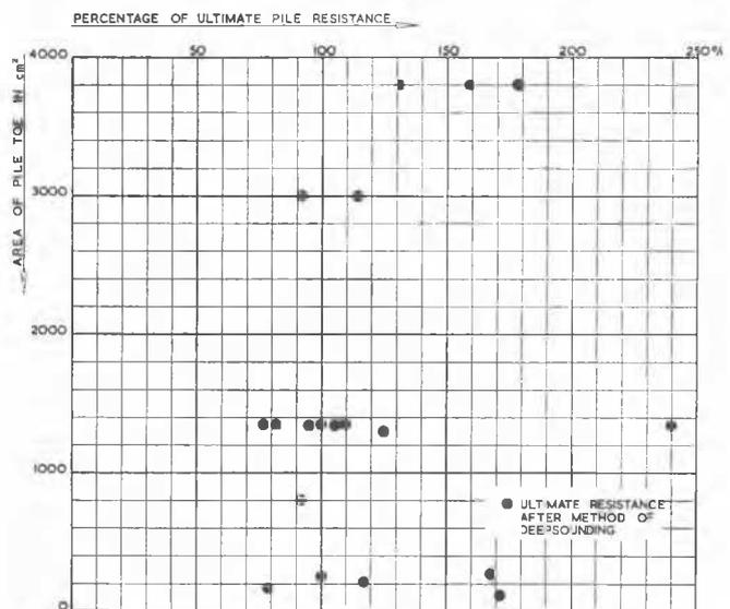
Fig. 11 Comparison of the Results of Loading-Tests and Deep-Soundings
