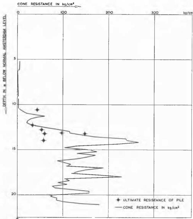
Fig. 10 Deep-sounding at Schiphol Airport, Amsterdam, with the Results of Some Loading-Tests
