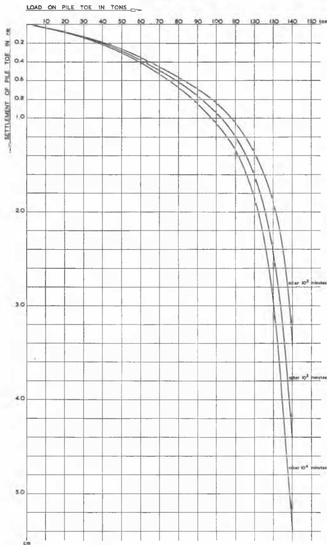
Fig. 7 Load-Settlement Curve of Concrete Pile No. 2, Slotermeer, at Different Time Intervals
