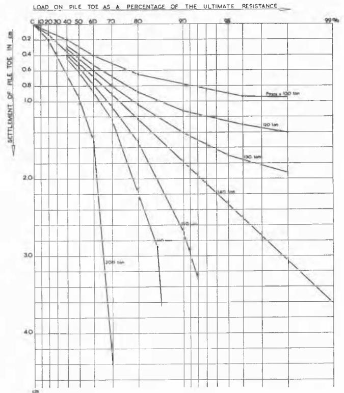
Fig. 4 Load-Settlement Curve of Concrete Pile No. 2, Slotermee, Drawn for Various Supposed Ultimate Resistances at Failure of the Pile
