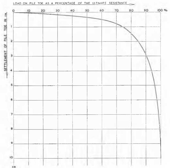
Fig. 2 Load-Settlement Curve of the *Plantema* Sounding Pile
