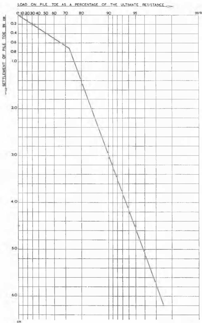
Fig. 3 Load-Settlement Curve of the *Plantema* Sounding Pile, plotted on a Semi-Logarithmic Scale
