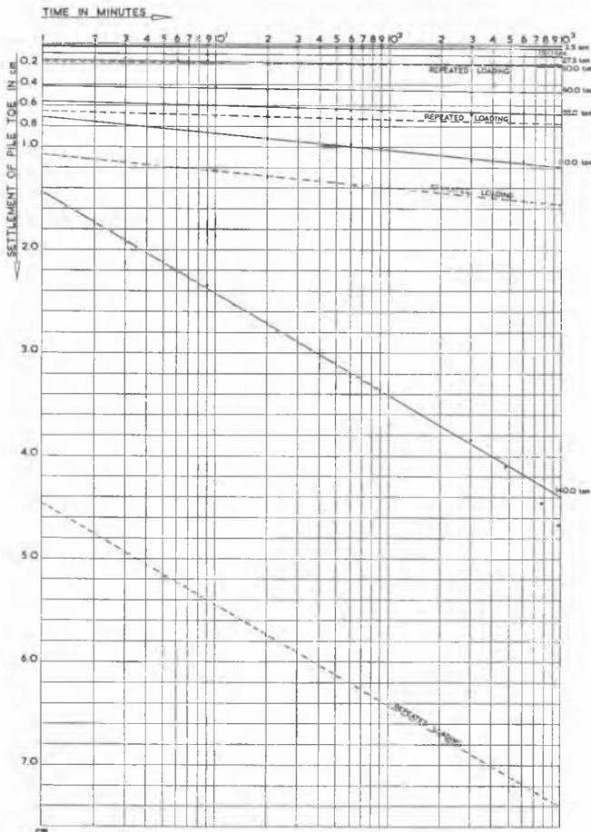
Fig. 6 Time-Settlement Curve of Concrete Pile No. 2, Slotmeer, Plotted on a Semi-Logarithmic Scale
