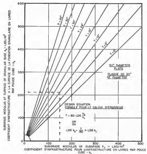
Fig. 12 Design Curves Giving the Value of the Subgrade Modulus  $k_b$  at the Surface of a Well Compacted Granular Base Course, when the Subgrade Modulus  $k_s$  of the Underlying Subgrade has been Measured
