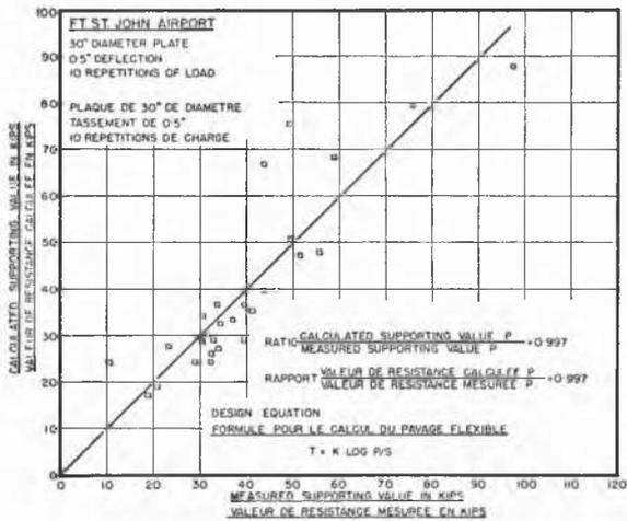
Fig. 7 Fort St. John Airport. Measured Runway Supporting Values Versus the Supporting Values Calculated by Means of the Flexible Pavement Design Equation
