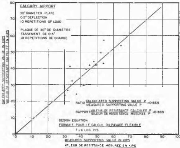
Fig. 8 Calgary Airport. Measured Runway Supporting Values Versus the Supporting Values Calculated by Means of the Flexible Pavement Design Equation
