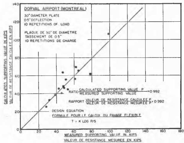
Fig. 6 Dorval Airport (Montreal). Measured Runway Supporting Values Versus the Supporting Values Calculated by Means of the Flexible Pavement Design Equation
