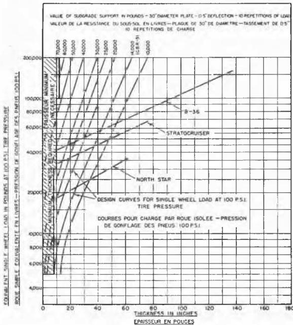
Fig. 2 Flexible Pavement Design and Evaluation Chart for Single-Wheel and Multiple-Wheel Landing Gear Assemblies (Tire Pressure 100 P.S.I.)
