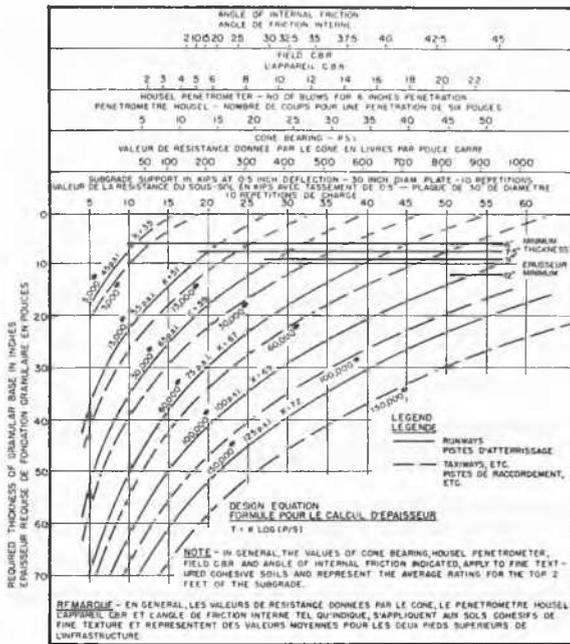
Fig. 1 Design Curves for Flexible Pavements for Runways and Taxiways, etc. for Aeroplane Wheel Loadings (Full Load on Single Tire)
