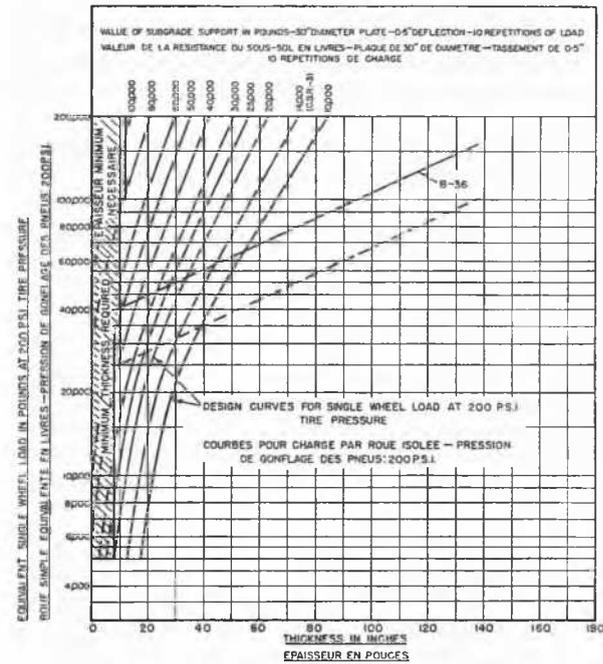
Fig. 3 Flexible Pavement Design and Evaluation Chart for Single-Wheel and Multiple-Wheel Landing Gear Assemblies (Tire Pressure 200 P.S.I.)
