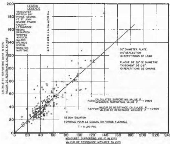
Fig. 11 Measured Runway Supporting Values Versus the Supporting Values Calculated by Means of the Flexible Pavement Design Equation for the Sixteen Airports for which these Data are Available
