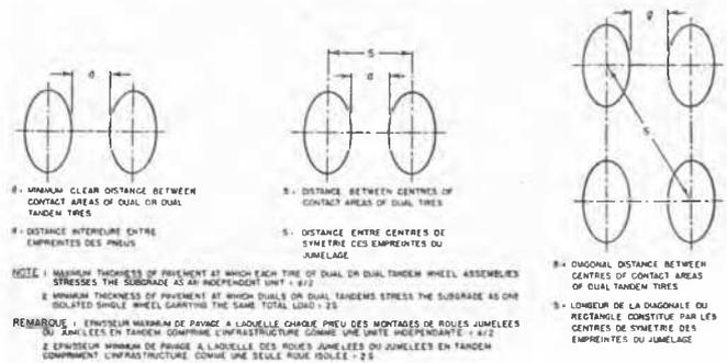
Fig. 4 Diagram Illustrating Dimensions of Contact Areas that Control Thicknesses of Pavements at which Dual or Multiple Wheel Assemblies Stress the Subgrade as Independent Units and as one Isolated Single Wheel Carrying the Same Total Load
