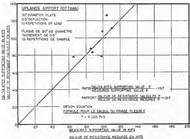
Fig. 5 Uplands Airport (Ottawa). Measured Runway Supporting Values Versus the Supporting Values Calculated by Means of the Flexible Pavement Design Equation
