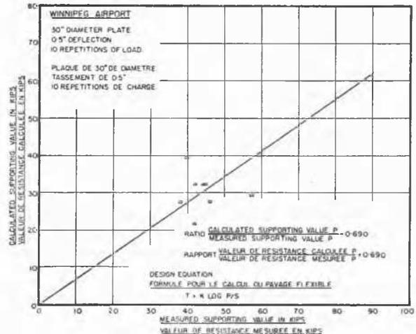
Fig. 10 Winnipeg Airport. Measured Runway Supporting Values Versus the Supporting Values Calculated by Means of the Flexible Pavement Design Equation
