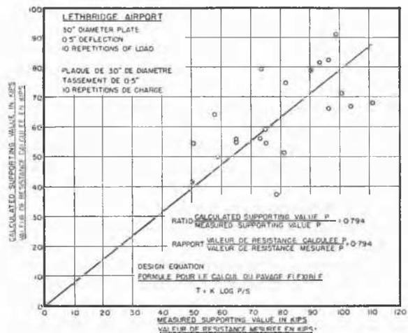
Fig. 9 Lethbridge Airport. Measured Runway Supporting Values Versus the Supporting Values Calculated by Means of the Flexible Pavement Design Equation
