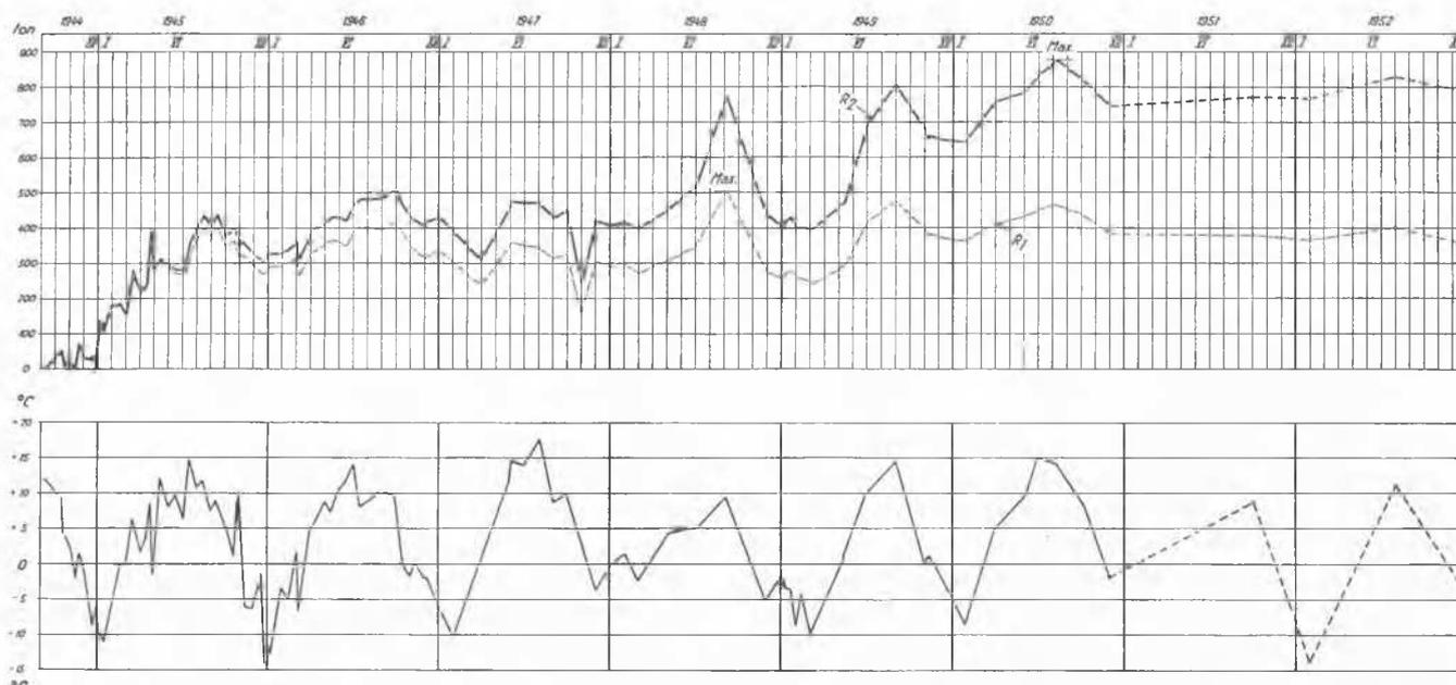
Fig. 7 Diagram of Measured Beam Pressure and Average Air Temperature. Curve  $R_1$  for a Variable Deformation Modulus  $V_b$  of the Concrete (Creeping) and Poisson Coefficient  $m = 5$ ,  $R_2$  for  $V_b = 200,000 \text{ kg/cm}^2$ ,  $m = 5$
