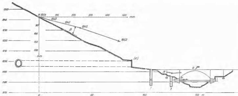
Fig. 5 True Displacement Vectors and Longitudinal Section ( $H-K-O$ , see Fig. 2)
