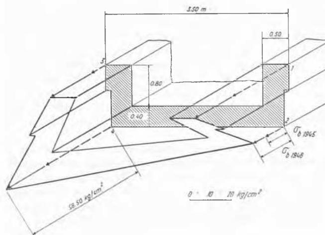
Fig. 6 Stress Distribution over the Cross Section of the Beam at the Moment of Maximum Pressure ( $V_b = 200.000\text{ kg/cm}^2$ ) August–September 1945 and 1948 (see Fig. 7)
