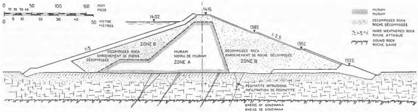
Fig. 2 Typical Cross-Section of the Earth Fill Section type
