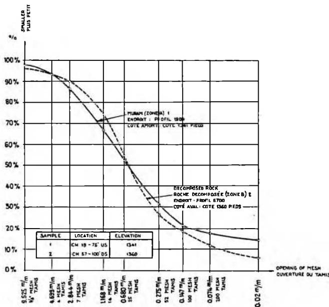
Fig. 3 Typical Grain Size Distribution Curves
