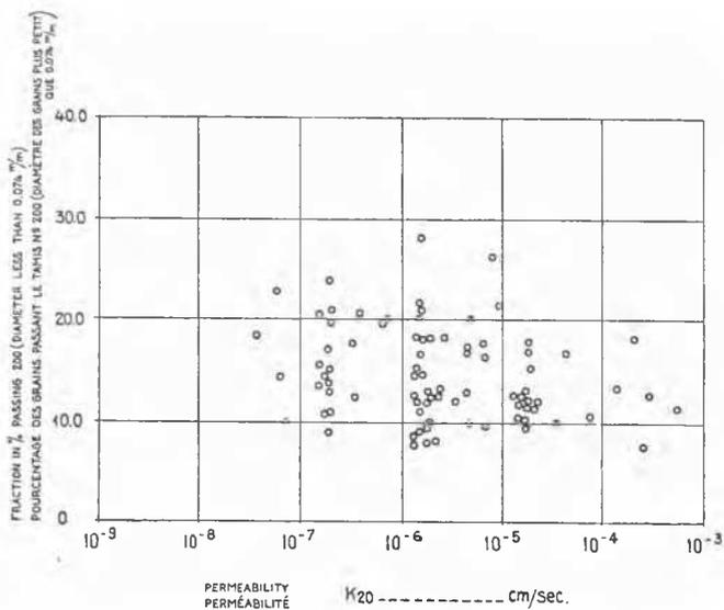
Fig. 4 Permeability of the Soils as Function of the Content of Fines
