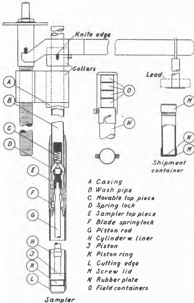
Combined sampler and loading tests cylinder
