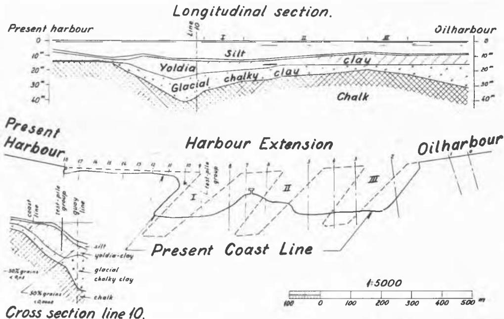
Plan of harbour extension with longitudinal and cross section.
