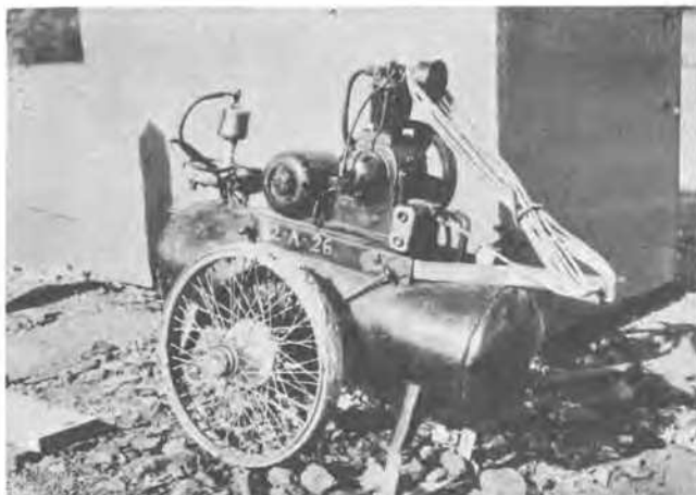
Portable Air-Compressor Unit.
