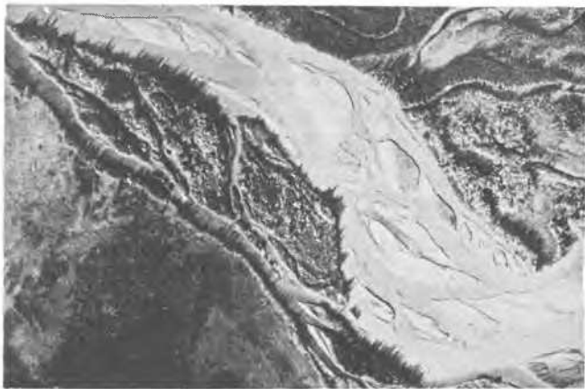
Airphoto pattern of a braided stream in a broad, silt-filled valley. In this instance permafrost prevails in the silt flood plains.
