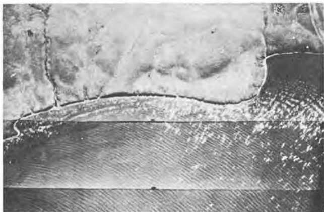
Intense polygon development indicating detrimental permafrost.
