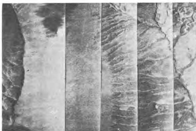
Contrasting airphoto patterns of contrasting soil types are illustrated in this photo. Two materials, upland residual soils and colluvial materials, are shown.
