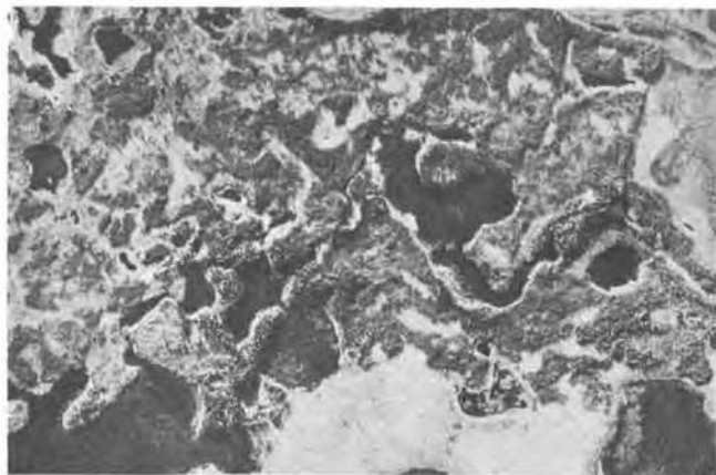
A typical airphoto pattern of a muskeg area in a broad, valley-fill region. The soils in this instance are frozen peat and silt.
