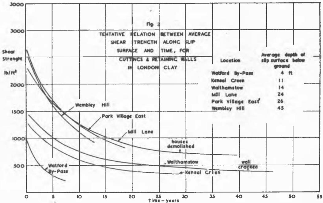
Tentative relation between average shear strength along slip surface and time, for cuttings & retaining walls in London clay.
